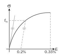
In case of brittle materials, offset method is used to find out the first crack in the material.
