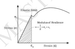
**Modulus of Resilience:** It is maximum strain energy stored in a material up to Elastic limit per unit volume.
