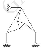
I. The truss is statically determinate II. The truss is kinematically determinate With reference to the above statements which of the following applies?
