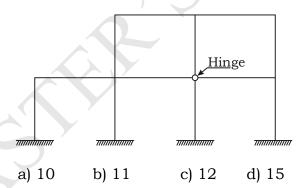
13. The degree of static indeterminacy for the rigid frame as shown below is
