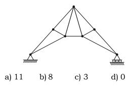
28. The degree of static indeterminacy of a rigidly jointed frame in a horizontal plane and subjected to vertical load only, as shown in figure below, is
