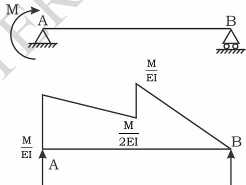
$$R_B \times l = \frac{1}{2} \frac{M}{EI} \times \frac{l}{2} \times \left( \frac{l}{2} + \frac{1}{3}l \right) + \frac{1}{2} \frac{M}{2EI} \times \frac{l}{2} \times \frac{1}{3} \left( \frac{l}{2} \right) + \frac{M}{2EI} \times \frac{l}{2} \times \frac{l}{4}$$
